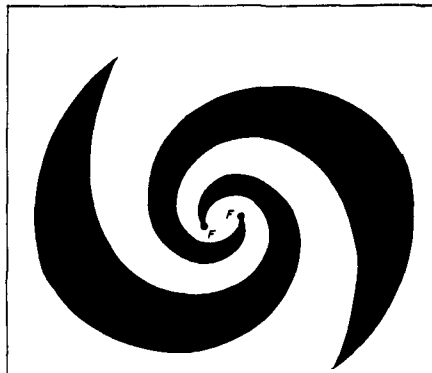
fig. 2. The two-arm equiangular dipole antenna is fed with a balanced line at F-F. The feedpoint impedance is relatively independent of frequency over operating range. Low frequency operating limit is defined by the circumference of antenna, indicated by the dashed line. (Drawing adapted from Jasik 2 .)
